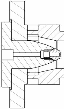
**Figure 4: Cross-section of the burner geometry**
