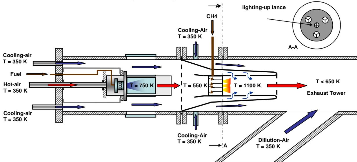
Figure 6: Schematic of the test cell and the afterburner
