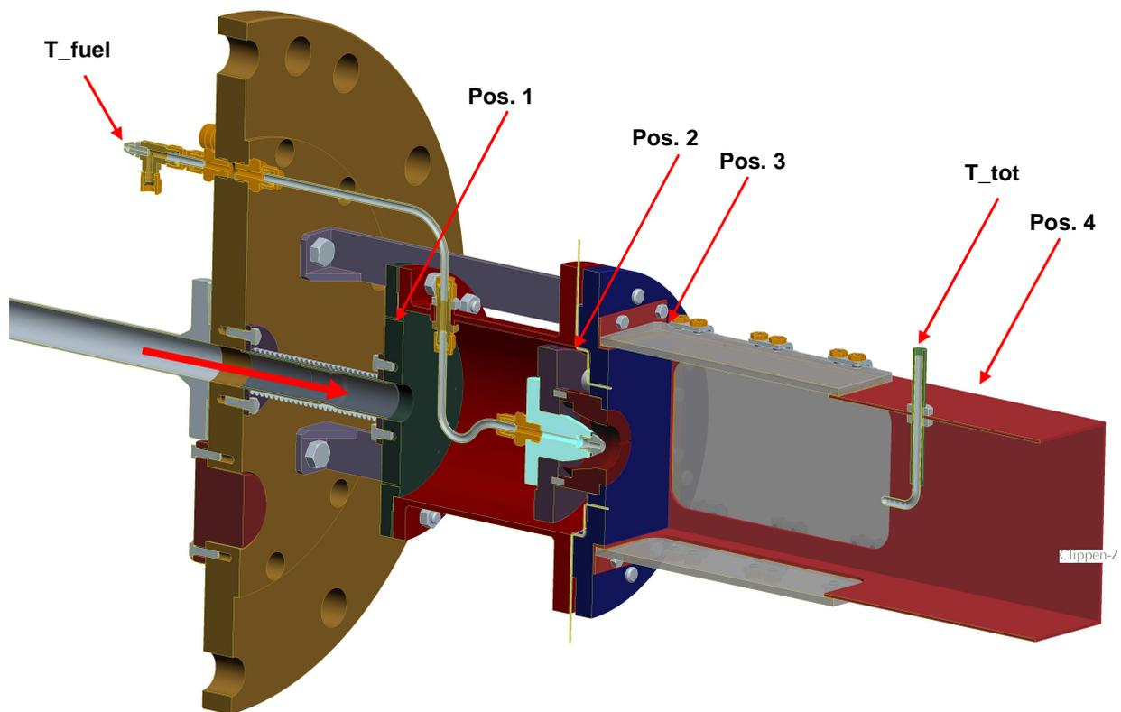
**Figure 5: Cross-section of the burner geometry**
