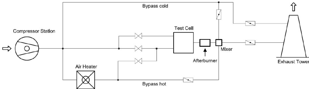
**Figure 1: schematic of the test facility**
