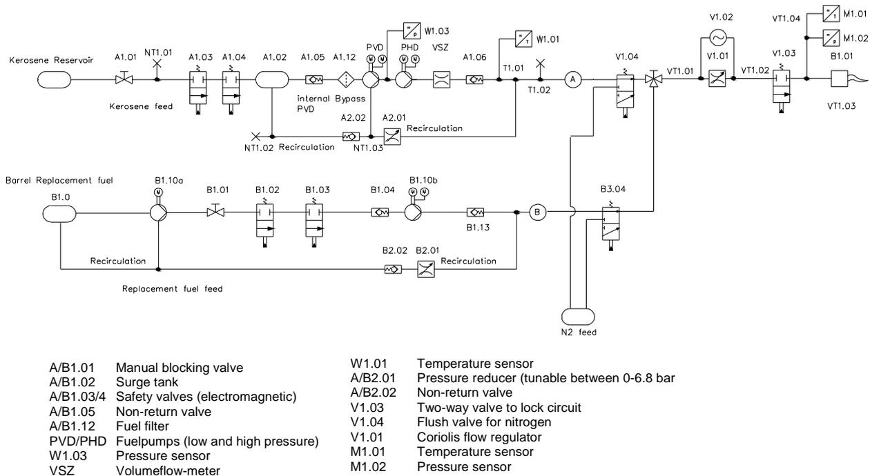
**Figure 3: Schematic of the fuel supply**
