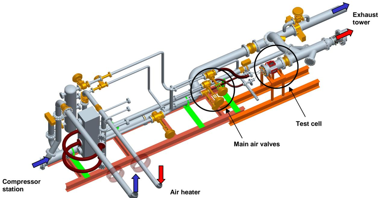
**Figure 2: 3D Design of the test facility [1]**
