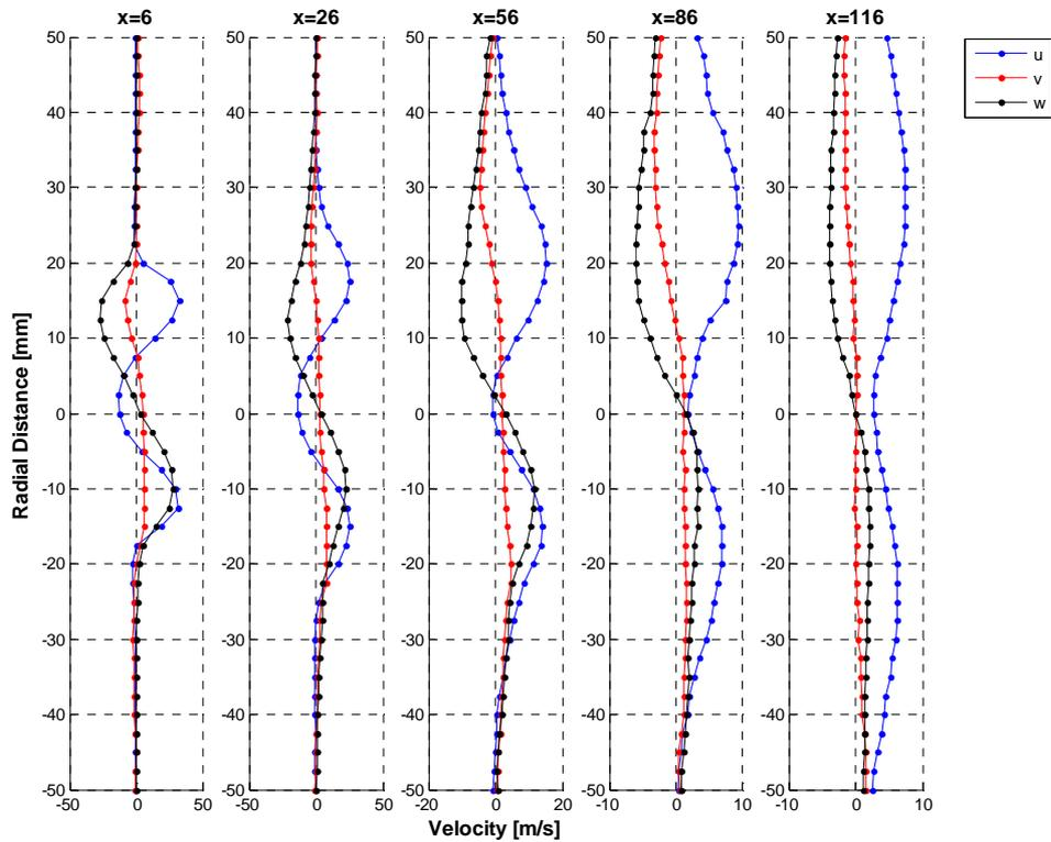
Figure 10: Radial-distribution of the velocity components  $u$ ,  $v$  and  $w$  in free-jet configuration
