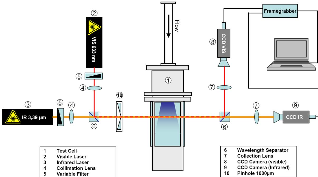
**Figure 7: IRE test configuration**
