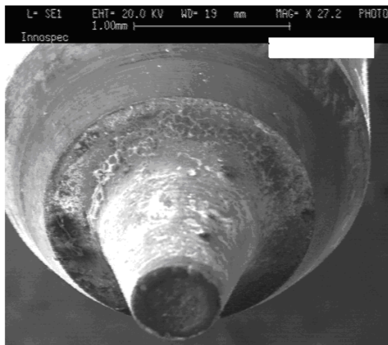
Figure 1 Typical fouled injector needle
