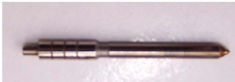
Figure 1 Typical fouled injector needle
