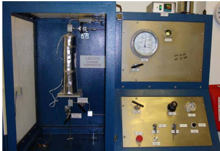
Figure 5 A Static rig capable of generating high pressures and temperatures
